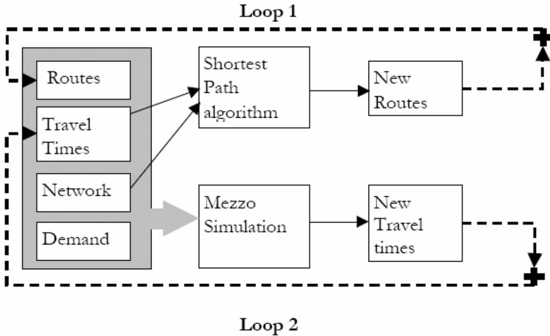
Figure 3.2: Iterative dynamic assignment procedure in Mezzo
