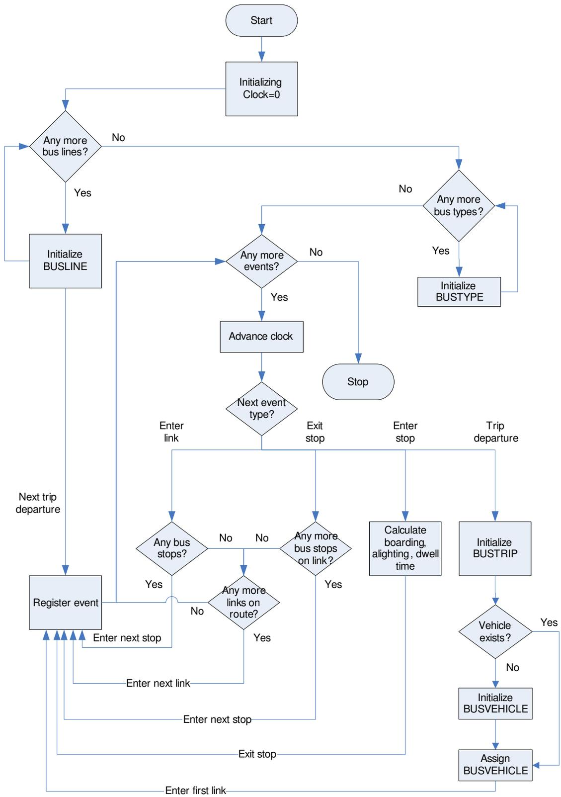
Figure 3.5: Flow Chart of the transit simulation process
